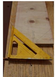
3. The top edge of the sides can have a 45-degree cut made to match the roof slope to fit tight. This is not necessary but may be an additional step desired for a fair project.
