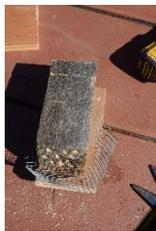
4. The roof of the house and bird guard are fastened to the house. The roof boards are put into place and the back screws (or air gun brads) are secured. Before the front screws (or air gun brads) are secured, the wire mesh bird guard must be cut and put in place. Woodpeckers have long bills and tongues so a guard must be placed across the entrance that is at least an inch away from the entrance.
