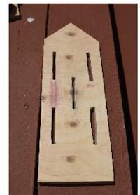
8. The slots can be cut with a router or using a drill and jigsaw. For jigsaw, a  $3/8$  wood spade or other drill bit is used to drill a hole on the marks of the slots. A pencil and straight edge is used to draw a line to guide the cut from the outer edges of the bottom hole to the outer edges of the top hole of each slot.
