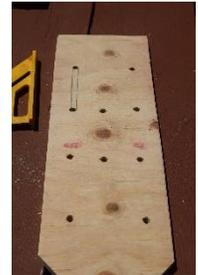
6. For the center slot, a mark is placed on the center of the width of the board and  $8\frac{1}{2}$  inches from the bottom. The top of the slot is measured at width midpoint and  $12\frac{1}{2}$  inches from the bottom.
