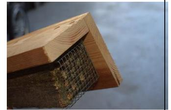
The mesh should be at least ¼ inch and stiff. The guard should be fitted to have top two edges under the roof and one edge long enough to staple a supported 3<sup>rd</sup> edge to the house. Once the guard is fitted to the house, the lip is tucked under the roof, formed and fastened. The guard needs to have about an inch of space from the screen to the entrance and the wire stiff to prevent the birds from compressing it.
