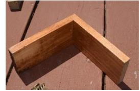
4. Next, the roof boards are cut for the peak. Each roof board peak is cut at a 45 degree angle so the roof boards fit tightly together at the top
