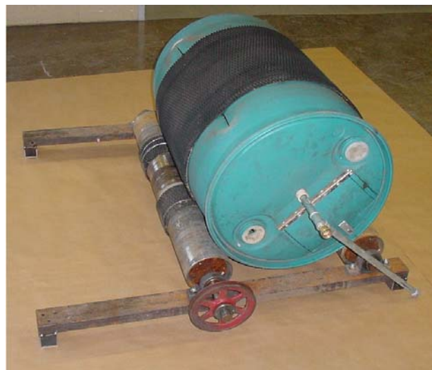
Figure 1. Assembled carrot washer (guard box and pulley guards not shown). Barrel rotation is clockwise to prevent movement of the stabilizer arm.
