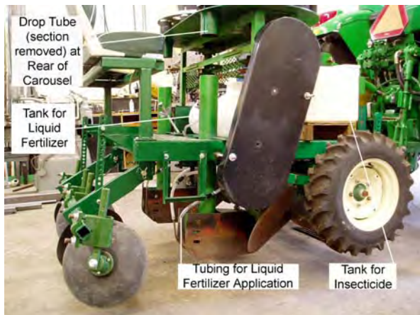
Figure 8. Side view of 2004 redesigned potato planter.
