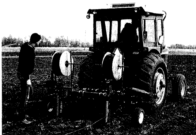
Figure 2—Installation of the subsurface drip irrigation tape.
