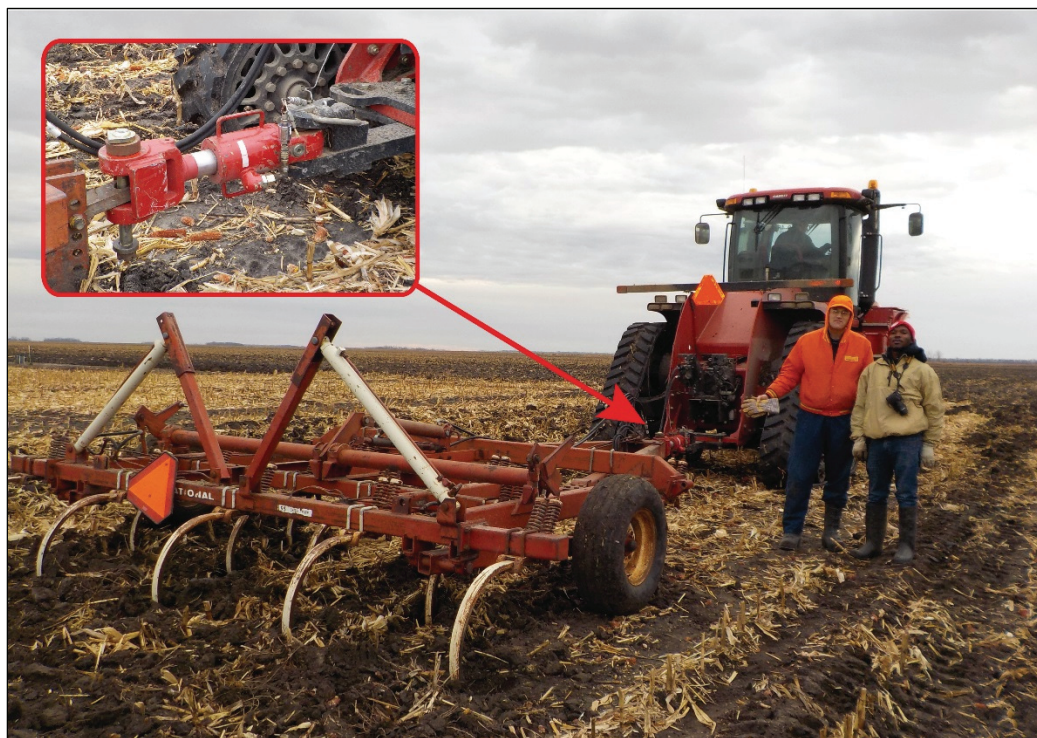
Figure 2. Tractor, pull meter, and chisel plow used to measure draft during tillage at an experimental field site near Wyndmere, North Dakota. The insert shows the pull meter used to measure draft on the chisel plow.
