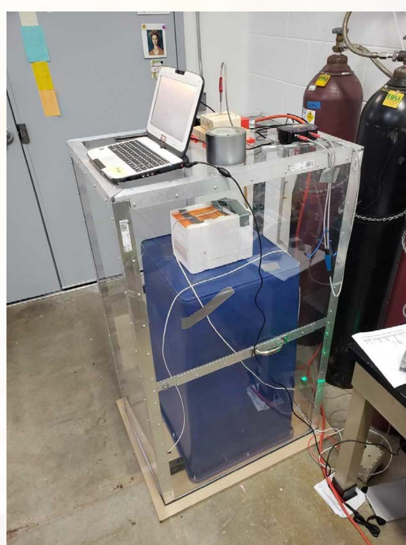
(Left) Shroud measuring oxygen levels of a mini-nuc.
