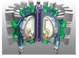
mak, where the fuels are injected into and confined in a vacuum chamber and heated to temperatures exceeding 100 million degrees Celsius. Under those conditions the fusion fuels become a gas-like form of electrically charged matter known as a plasma. (Its electric charge is what allows confinement by magnetic forces.) ITER will test the ability of magnetic confinement to hold the plasma in place at high enough temperatures and density for a long enough time for the fusion reaction to take place.
