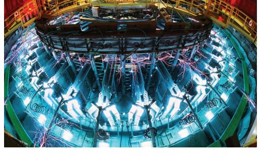
Sandia National Laboratories' Z machine uses the inertial confinement method to heat and fuse pellets of hydrogen.
