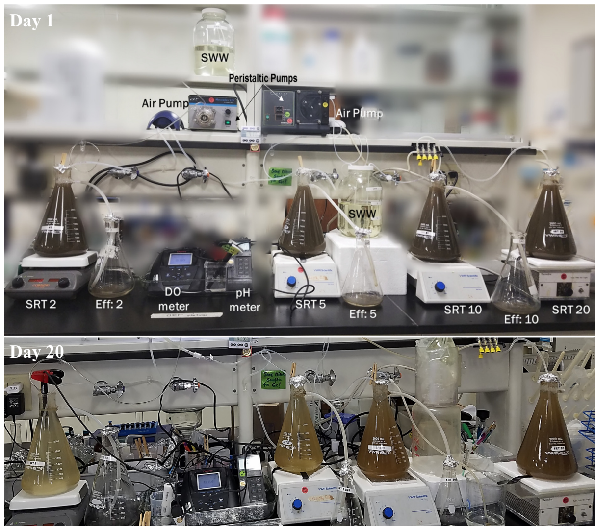
Fig. 1. Bench-scale experimental setup for chemostat operation on day 1 (top) and day 20 (bottom). SWW – synthetic wastewater water; Eff – effluent; SRT – solids retention time.
