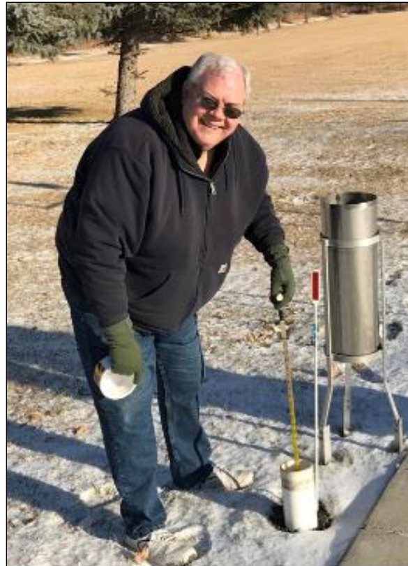
NWS Grand Forks ND Observation Program Lead (OPL), Brad Hopkins, takes a frost depth reading using a frost tube. NWS photo.
