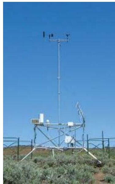
Figure 14. A typical RAWS station. Image courtesy of the USDA, National Wildfire Coordinating Group.
