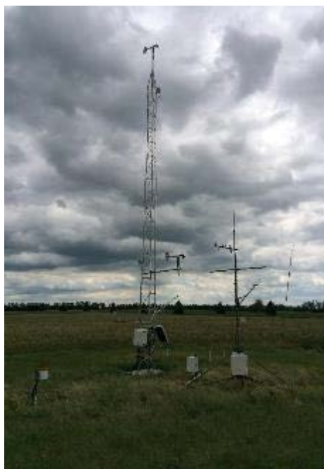
Figure 15. The NDAWN station located at Carrington 4N. Note the impeller type wind sensors located at 3 and 10 meters high on the tower. Image courtesy of the North Dakota Ag Weather Network.
