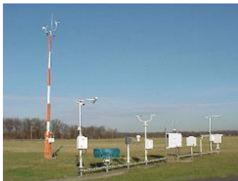
Figure 13. An Automated Surface Observing System (ASOS) at an airport. The 10 meter tower hosts a wind vane and anemometer. Image courtesy of
