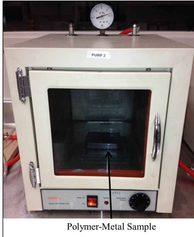
Figure 27: Adhesive sample curing in a vacuum-furnace
