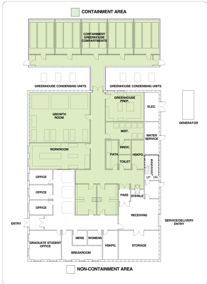
FIGURE 7. Typical Containment Facility Floor Plan*
