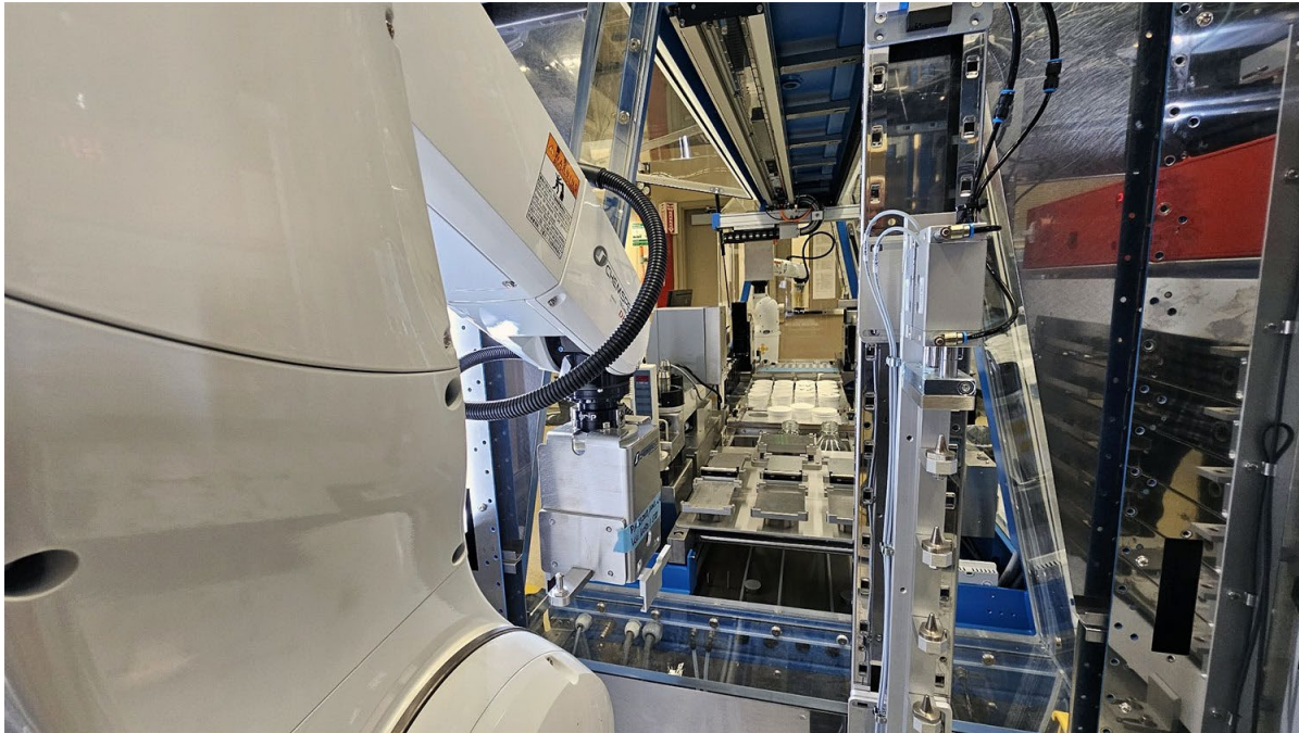
The NDSU combinatorial Materials Research Laboratory (CMRL) utilizes an automated approach with robotic systems to rapidly synthesize and test large libraries of diverse materials
