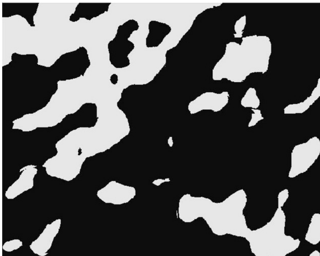
Figure 5-10. Layered and clustered map of Thomasboro with EM readings combined with elevations. This map was developed using the same procedure as explained in Figure 5-9.
