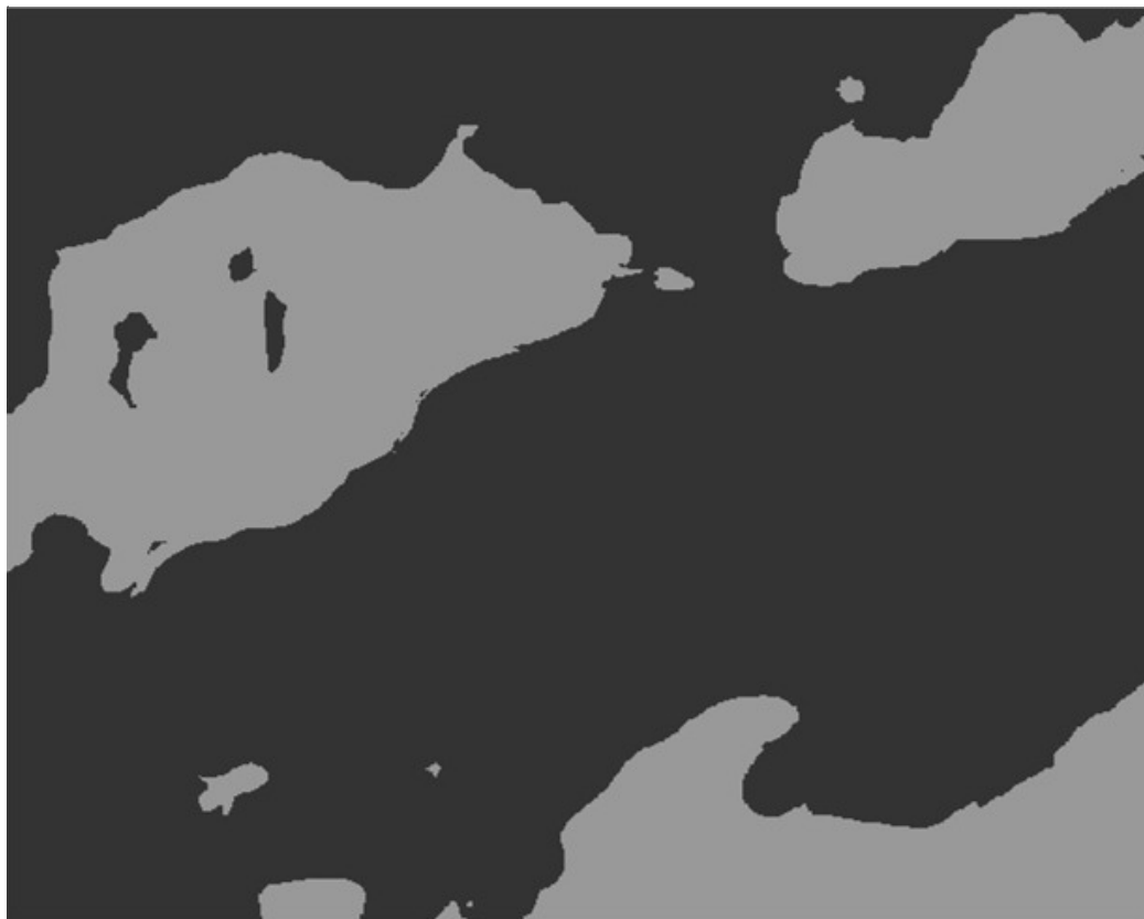
Figure 5-9. Layered and clustered zones derived from elevations and EM readings, Mansfield. This image was derived using a combination of ArcMap to register the elevation and EM maps, then was imported into ERDAS Imagine as a .img file. The files were layered and the layers were subjected to unsupervised classification using the isodata clustering method embedded within Imagine. This map shows the higher landscape positions being segregated from the rest of the field.
