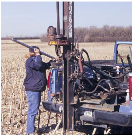
Figure 6. Use of a pickup bed hydraulic system in the field to sample deep depths.
