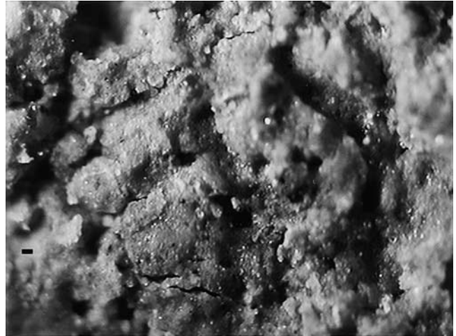
Fig. 7. Continuous thick clay films from the 55- to 58-cm depth (2Bt horizon) in Pedon 40 (scale bar = 200 \mu\text{m} ).
