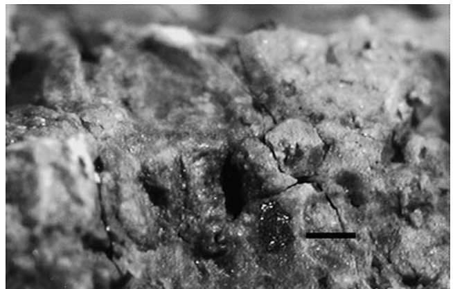
Fig. 8. Fine sand grains enveloped in continuous thick clay films from the 65- to 69-cm depth (2Btk1 horizon) in Pedon 40 (scale bar = 200 \mu\text{m} ).
